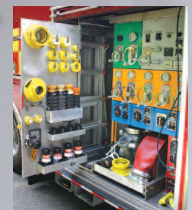
Customized storage for pump accessories.
