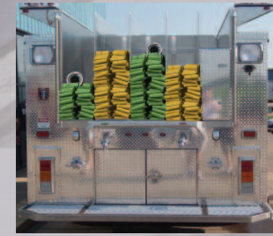
The Star Series is all about usability. The unique shape of the form-fitted tank allows for an extremely low hose bed.
