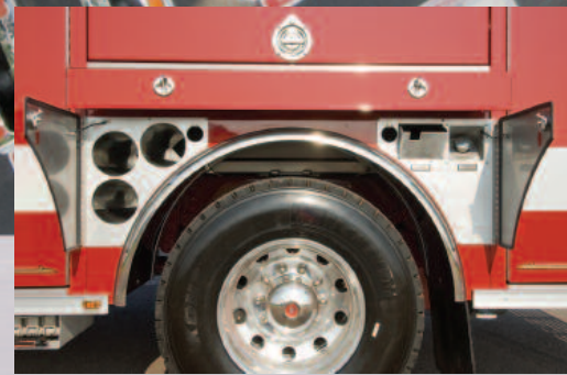
Optional storage around the wheel wells increases the amount of usable compartment space. The Smart Storage compartments were designed to free up body compartment space and bring equipment to a more usable height.
