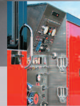
The Smart Display Pump control panel option is angled from the top for better visibility and reduced glare.
