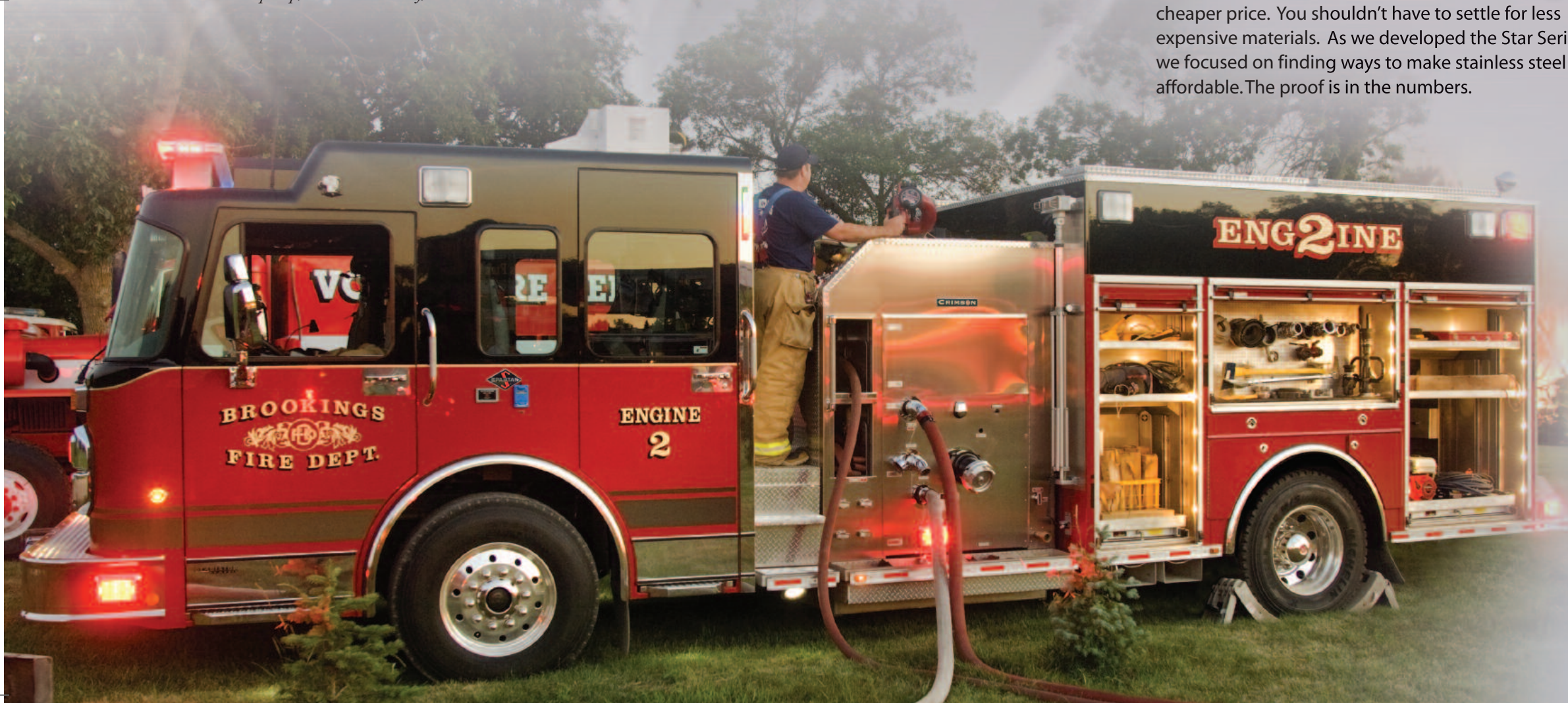
The Crimson Star Series Pumper Shown with a midmount pump, custom built body, and custom chassis.
