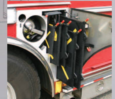
Customized Smart Storage capable of housing up to 7 air bags and a 2 1/2 gallon water extinguisher.
